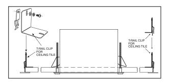
d. Install the ceiling tile with the back box. Attach a T-rail clip on each side of the ceiling tile. Fasten the L-bracket to the clip with the supplied screw and washers. e. Attach the wiring to the circuit board inside the back box. When finished, close the door to the back box and turn on the power. The red LED will light.
